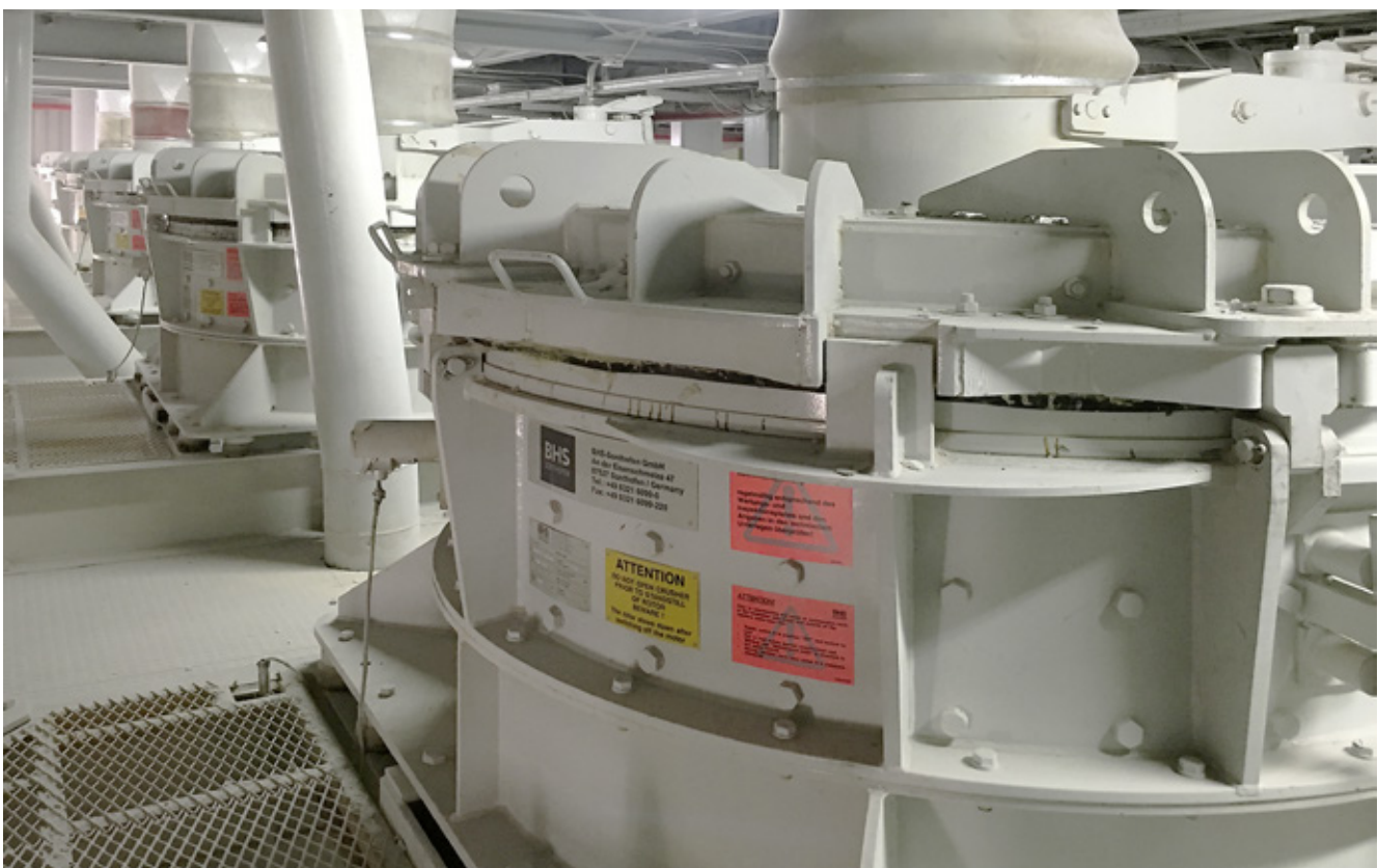
Five BHS rotor impact mills of the RPM 1513 type are in use at a dry-mortar plant in Thailand
