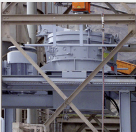
RPM 1113 for the production of high-quality crushed sand (0–2 mm) from off-spec gravel fractions (2–5 mm, andesite)
